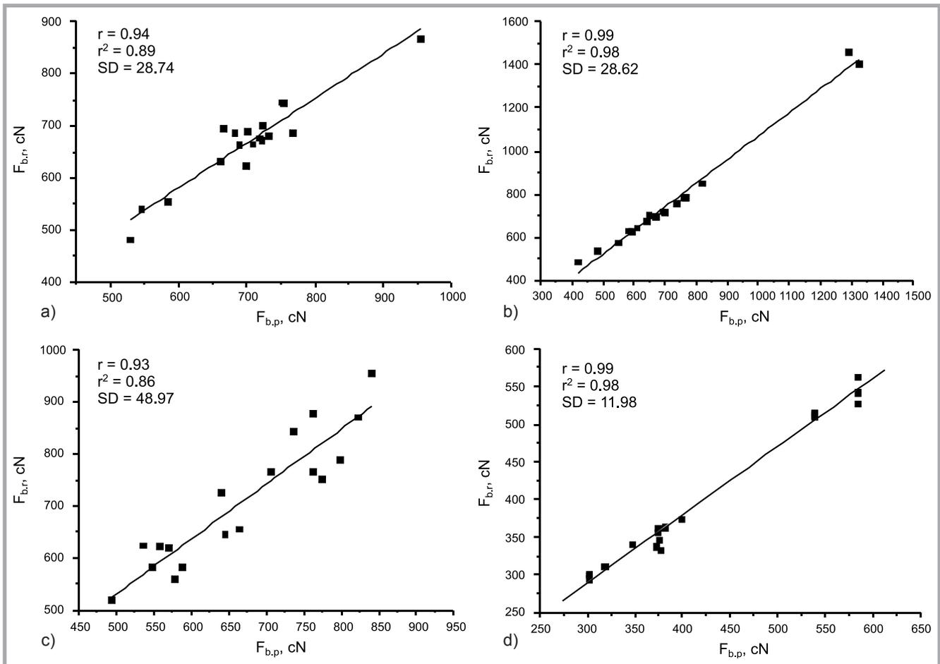
**Figure 4.** Correlation of projected and real breaking force values of: a) single ring-spun and twisted yarns (1 to 18), b) single rotor and twisted yarns (19 to 36), c) single and twisted yarns (37 to 54), d) single and twisted yarns (55 to 72).
