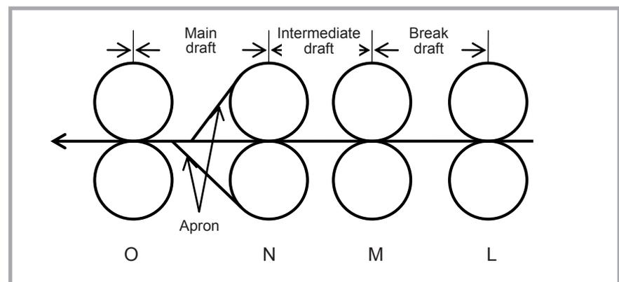
*Figure 1.* Drafting arrangement of vortex spinning.
