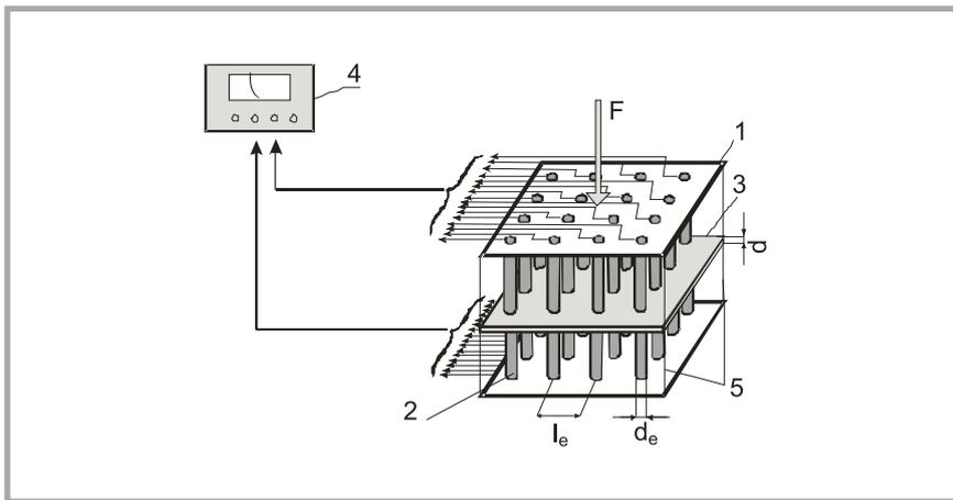
**Figure 5.** Simplified scheme of the volume resistance measurement stand, 1 – upper multipoint measurement probe, 2 – lower multipoint measurement probe, 3 – textile electrode, 4 – Agilent 6.5 Digits Mullimeter, 5 – crossrails,  $F$  – preasure force
