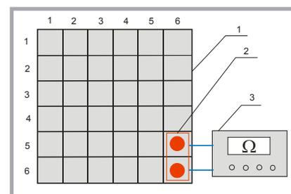
**Figure 4.** Simplified scheme of a stand for measuring surface resistance; 1 – textile electrode, 2 – dual point probes, 3 – Agilent 6.5 Digits Multimeter.
