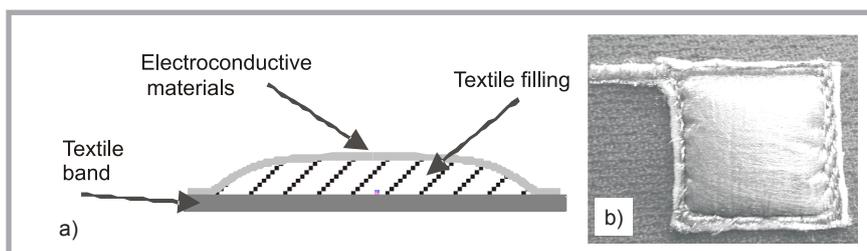
**Figure 1.** Scheme of a textile composite electrode for electrostimulation (a), real photo of the structure (b).
