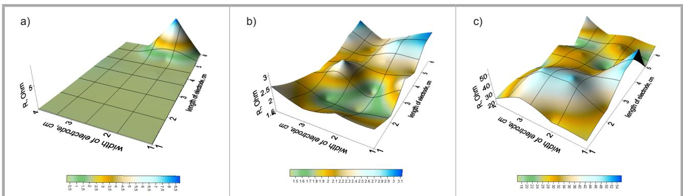
**Figure 6.** Example of the surface resistance distribution on a textile electrode: 1 – electro-conductive silicone foil with silver particles, 2 – woven fabric made of Nitril Static yarn, 3 – graphite nonwoven.
