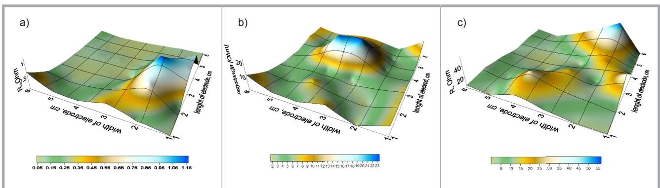
**Figure 7.** Example of the volume resistance distribution on a textile electrode: 1 – electro-conductive silicone foil with silver particles, 2 – woven fabric, made of Nitril Static yarn, 3 – graphite nonwoven.
