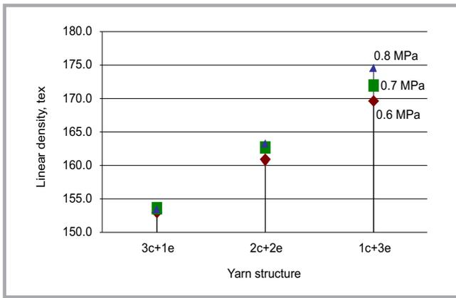
**Figure 1.** Dependence of yarn linear density on the structure of the yarn.
