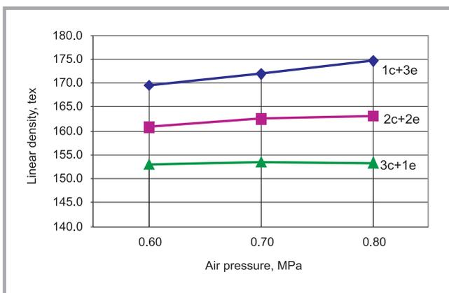
**Figure 2.** Dependence of yarn linear density on air pressure.
