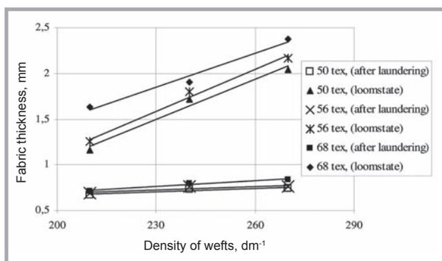
**Figure 6.** Thickness variation of fabric and increasing density of wefts when linear density of wefts is constant.
