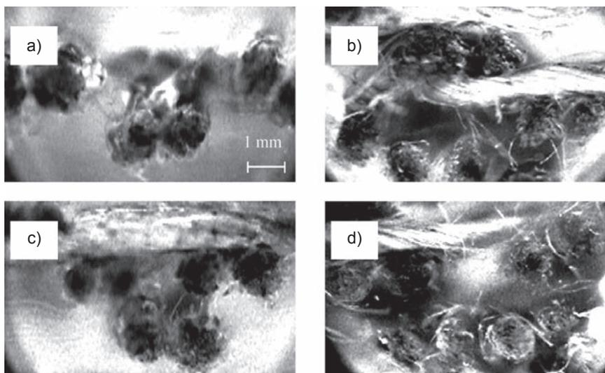
**Figure 5.** Cross-sections of fabrics from 56 tex linen spun yarns: (a) loomstate fabric, with  $S_2 = 210 \text{ dm}^{-1}$ , (b) fabric after laundering, with  $S_2 = 210 \text{ dm}^{-1}$ , (c) loomstate fabric, with  $S_2 = 270 \text{ dm}^{-1}$ , (d) fabric after laundering, with  $S_2 = 270 \text{ dm}^{-1}$ .
