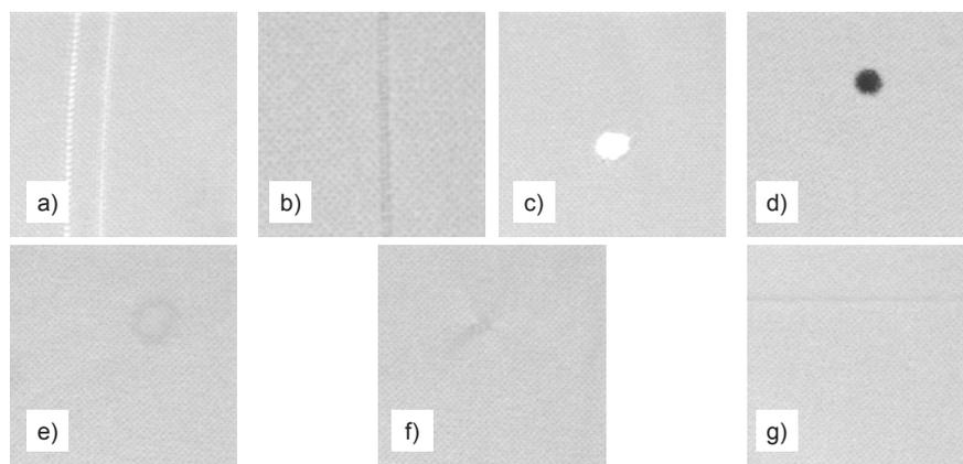
**Figure 1.** Seven fabric defects; a) Laddering, b) End-out, c) Hole, d) Oil spot, e) Dye stain, f) Snag, g) Crease mark.
