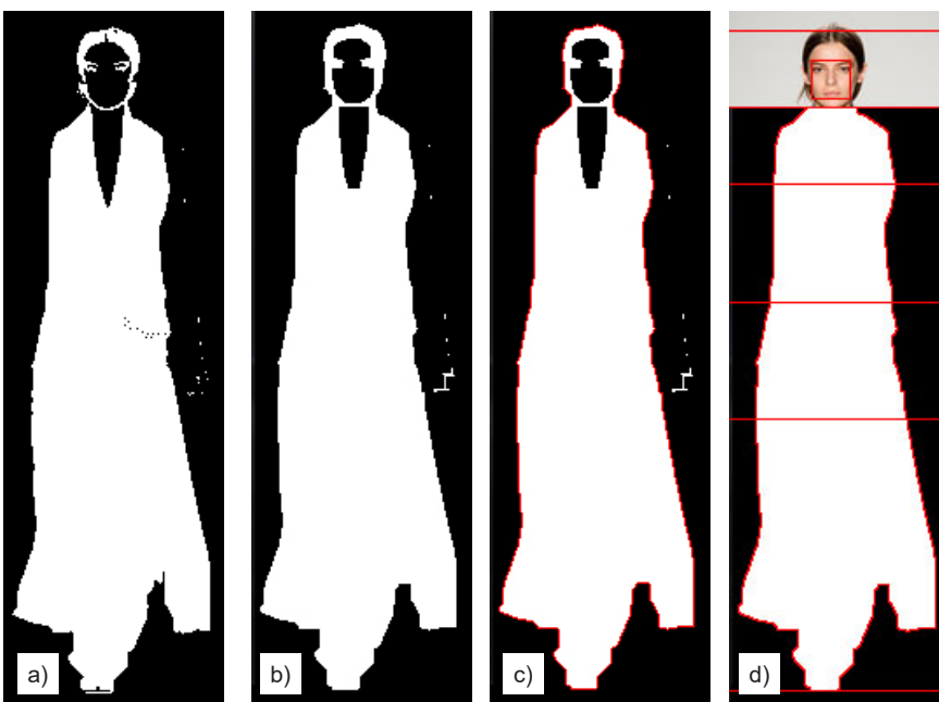
Figure 9. Major steps in image processing. a) OTSU thresholding, b) Morphol. Operation, c) Contour tracing, d) Body division.
