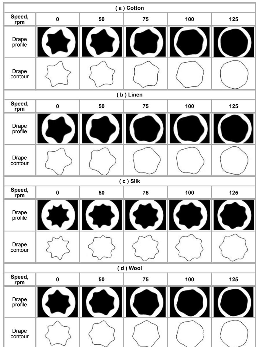
Figure 3. Typical dynamic drape profiles and their contours after an image processing of the fabrics at rotating speeds of 0, 50, 75, 100, and 125 r.p.m.
