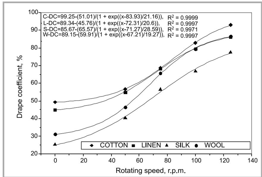
Figure 4. The relation of the drapability coefficient to the rotating speed. Line drawn through the experimental points is a Boltzmann fit.
