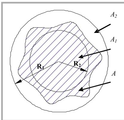
**Figure 2.** Definition of the fabric drape coefficient;  $A$  - actual projected area of specimen,  $A_1$  - area of supporting disk,  $\pi R_2^2$ ,  $A_2$  - area of specimen,  $\pi R_1^2$ ,  $R_1 = 15\text{cm}$ ,  $R_2 = 9\text{cm}$ , Drape coefficient =  $(A - A_1)/(A_2 - A_1)$ .
