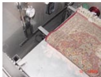
Figure 2. Typical photos of the simulator apparatus to measure the compression creep behaviour of carpet.
