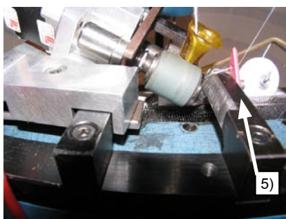
Figure 4. Peculiarities of the feeding device; 1 – feeding device, 2 – funnel guide, 3 – sensor of open needles, 4 – sensor of loops not worked-in, 5 – guides for filaments, 6 – working region.
