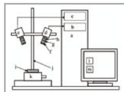
Figure 1. Measurement system: a) PC computer, b) video card No.1, c) video card No.2, d) video camera No.1, e) video camera No.2, f) focus setting, g) zoom setting, h) diaphragm setting, i) sample of tested material, j) stand, k) micrometrical table with light, l) Textil2D application, m) application Loo2D application.
