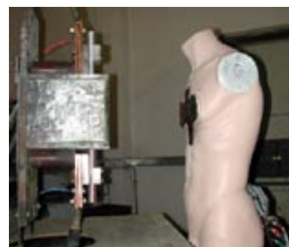
Figure 6. Test mannequin with calorimeters in the chest area (Method 2).
