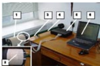
View of the TEXTILPRESS measuring stand during measuring; 1 – textile compression band, 2 – measuring matrix placed under the band, 3 – cylinder, 4 – cylinder holder, 5 – data acquisition system, 6 – computer.
