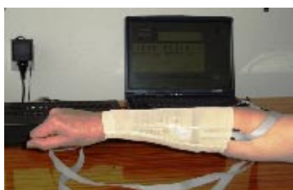
Measurement of the pressure exerted by a compression band with the use of the TEXTILPRESS device.
