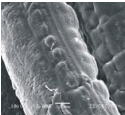
Figure 12. SEM micrograph of the surface chitosan fibres at temperature 70 °C (sample N C13), magnification 3000 \times .
