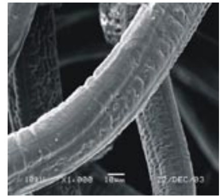
Figure 11. SEM micrograph of the surface chitosan fibres at temperature 70 °C (sample N C13), magnification 1000 \times .
