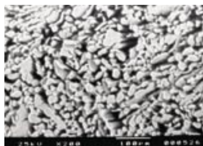
Figure 5. Cross-sections of the flax fibers after biological modification.
