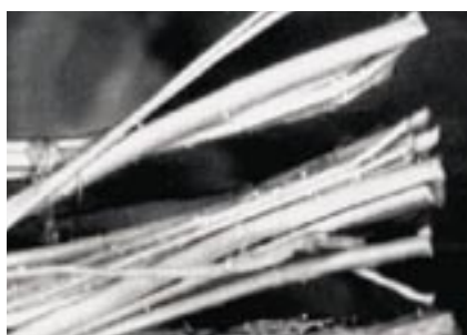
Figure 4. The surface of the flax fibers after biological modification.
