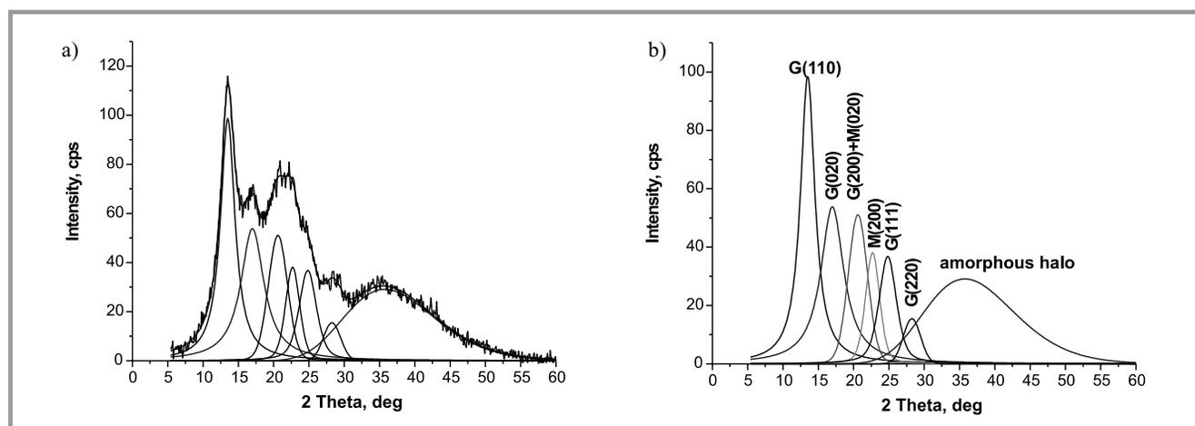
**Figure 4.** An example WAXS curve for a sample of alginate filament (fibres precipitated in the coagulation bath without  $\text{CaCl}_2$ ) a) curve resolved into individual peaks, b) diffraction reflexes with adequate Miller indices.
