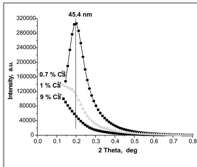
**Figure 6.** The comparison of SAXS curves (in the direction parallel to the fibres' axes) for alginate filaments with the different  $\text{Ca}^{++}$  ion content.
