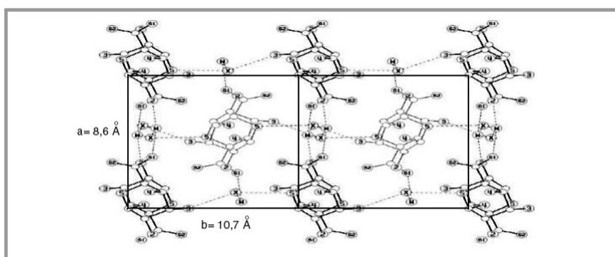
**Figure 3.** View of the crystal structure of hydrated guluronan the  $c$  axis projection of two complete unit cells with a vertical, the central diamond shows all the  $\text{O}\cdots\text{water}\cdots\text{O}$  bridges that glue the matrix together - the  $\text{O}61\cdots\text{W}\cdots\text{O}2$  bridges vertically and the  $\text{O}3\cdots\text{X}\cdots\text{O}5$  bridges horizontally.
