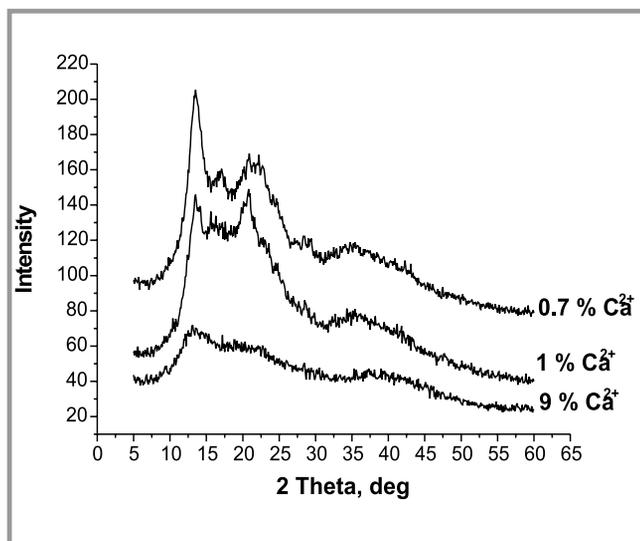
**Figure 5.** WAXS curves for alginate filaments with the different  $\text{Ca}^{++}$  ions content (fibres formed in coagulation baths with the different concentration of calcium chloride).
