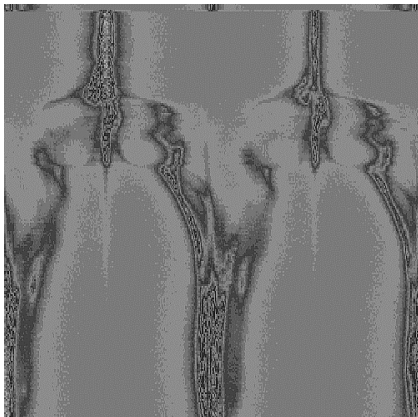
Figure 4. The position and intensity of the liquid crystal domains after a rotation over 90°. The vertical axis is the time axis, and the horizontal one the angular position from 0 - 360°. The way the data was derived is described in the text above.
