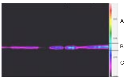
Figure 3. Thermogram with separated warp feeding, knitting and fabric take-up zone: A - warp feeding zone, B - knitting zone, C - take-up zone of the knitted fabric. Remark: This figure is presented in colour in the internet - edition of the journal ( www.fibtex.lodz.pl )
