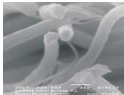
Figure 1. PAN fibre precursor nonwoven and fibre cross-section image, SEM microphotograph.
