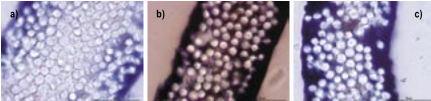
Figure 2. A view (POM) of cross-sections of composites based on: a - friction yarn, b - twisted yarn, c - textured yarn.
