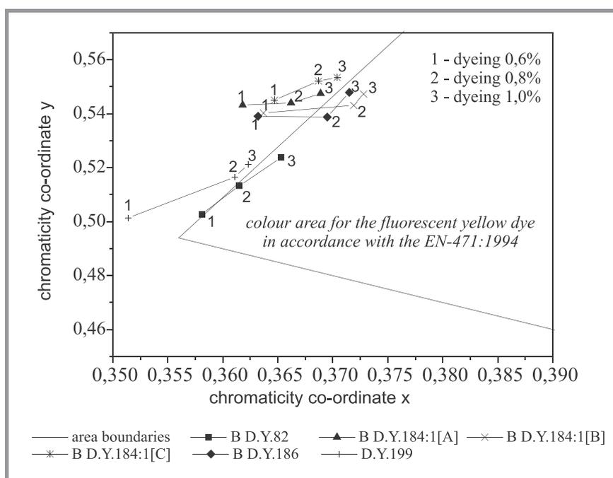
Figure 3. The chromaticity parameters of the dyeings of 0.6%, 0.8%, and 1.0% colour strength presented in the x-y chromaticity co-ordinates, in relation to the area boundaries for the fluorescent yellow dye in accordance with the EN-471:1994 standard.
