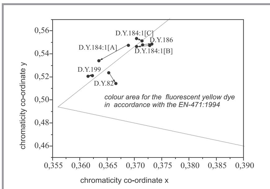
**Figure 5.** Colour differences of dyeings carried out with the use of the dyes tested before and after illumination of the samples in the Xenotest apparatus, presented in the x-y colour co-ordinates.
