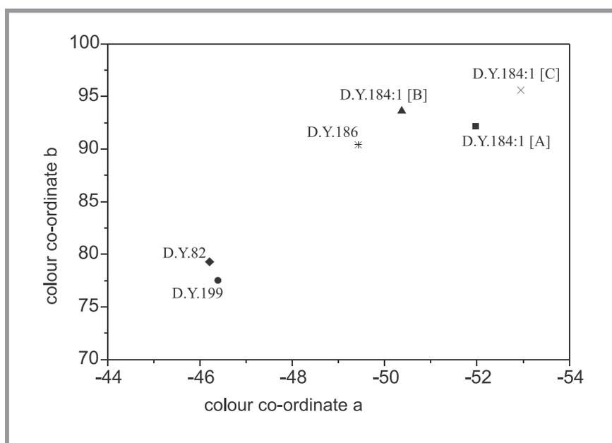
Figure 2. The colours of dyeings carried out with the use of fluorescent disperse dyes presented in the CIE chromaticity diagram in the a-b rectangular co-ordinates.
