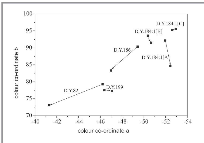
**Figure 4.** Colour differences of dyeings carried out with the use of the dyes tested before and after illumination of the samples in the Xenotest apparatus, presented in the a-b colour co-ordinates; \*the arrows indicate the directions of the position displacements for the individual sample colours within the a-b co-ordinates after sample illumination.
