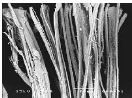
Figure 3. Surface of a hemp fibre after biological modification, variant IV.
