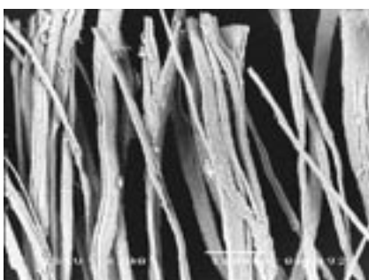
Figure 7. Surface of modified hemp fibre after carding, variant IV.
