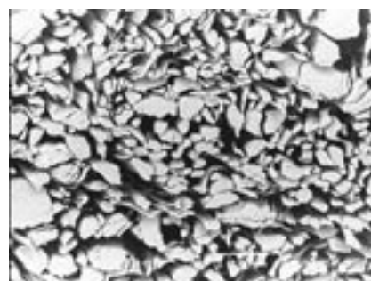
Figure 8. Cross-section of modified hemp fibre after carding, variant IV.
