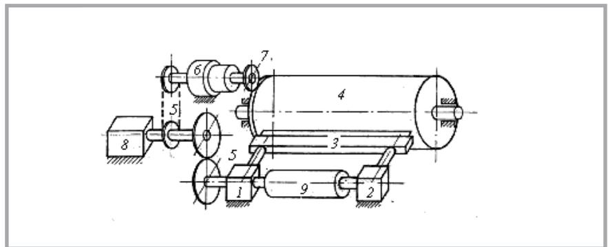
**Figure 1.** Loop-forming device of Kinemat 200; 1, 2 - loop-forming mechanisms, 3 - pushing ruler, 4 - loop-forming drum, 5 - teeth-chain reducer, 6 - wave reducer, 7 - gear train, 8 - electrical motor, 9 - flywheel.
