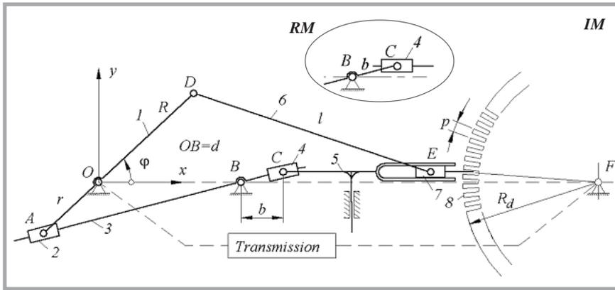
**Figure 2.** Ideal (IM) and real (RM) loop-forming mechanism; 1,6,7 - slider-crank mechanism; 1,2,3 - crank-shaper mechanism; 3,4,5 - tangent mechanism (IM) or cosine mechanism (RM); 7 - slider; 8 - loop-forming drum.
