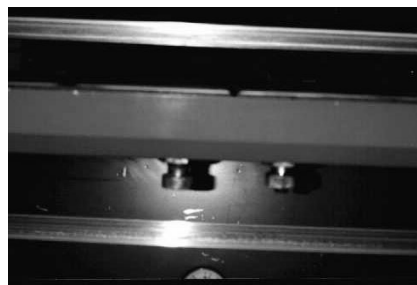
Figure 2. Fibre breaking in the first zone (B) of preliminary breaking; breaking by fibre bundles occurs only to a minimal degree.
