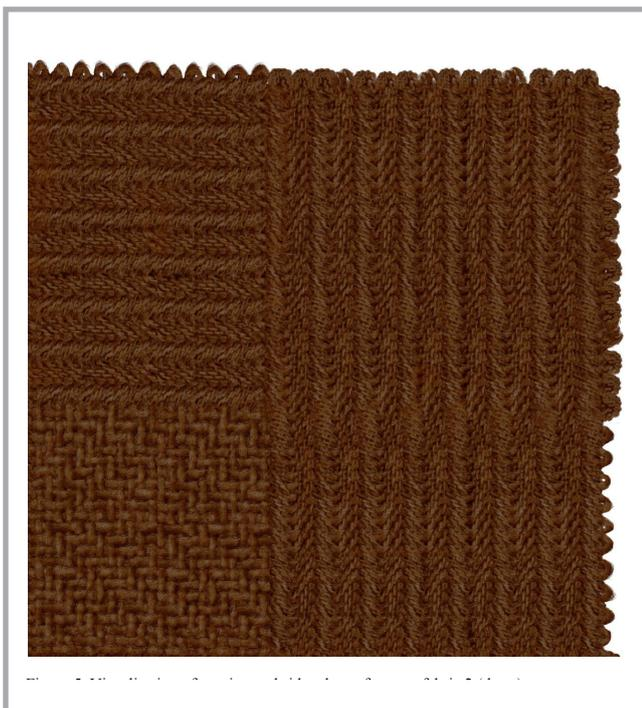
**Figure 5.** Visualisation of starting and side edges of woven fabric 2 (dress).
