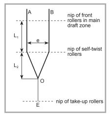
**Figure 1.** Schematic diagram of self-twist spinning process. Where:  $L_1$  – distance from the nip of front rollers to the nip of self-twist rollers,  $L_2$  – distance from the nip of self-twist rollers to the convergence point O, O – convergence point of strands A and B, e – distance between two strands.
