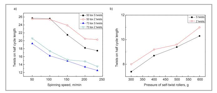
*Figure 4.* Twists over the half cycle length with the spinning speed and the pressure of the self-twist rollers: a) twists over half cycle length and spinning speed, b) twists over half cycle length and pressure of self-twist rollers.
