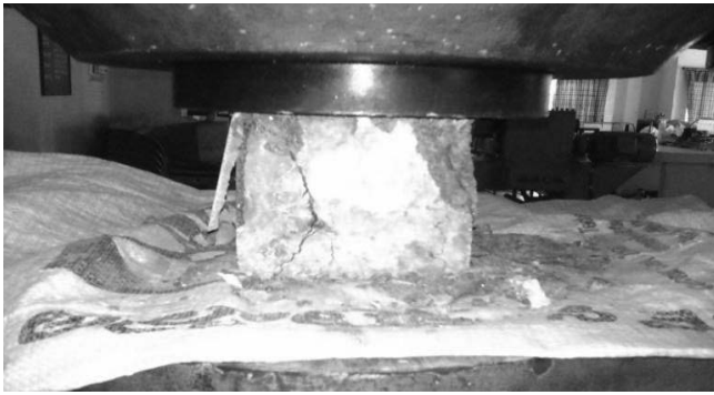
Figure 1. Failure of cube under compression.
