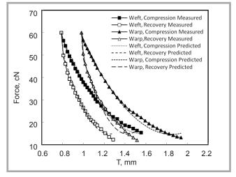
*Figure 4.* Comparison of theoretical and experimental results for sample 2.
