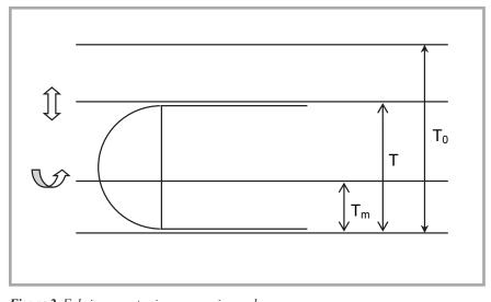
Figure 1. Rheological model for bending of fabric.
