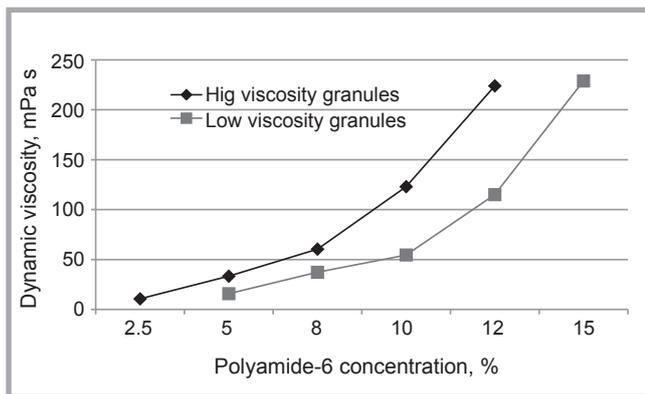
**Figure 2.** Influence of polyamide-6 concentration on dynamic viscosity of spinning solutions.
