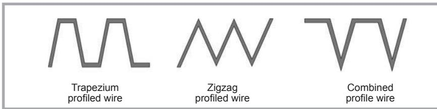
Figure 1. Different profiled wires for realization of the MWSF structure.
