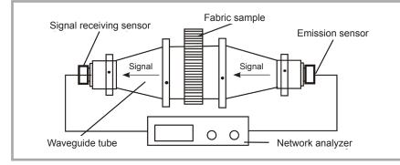
Figure 2. Schematic diagram of waveguide testing system.
