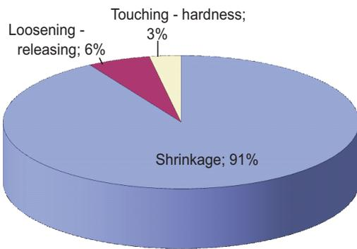
Figure 11. Possible issues experienced in the cutting procedure.
