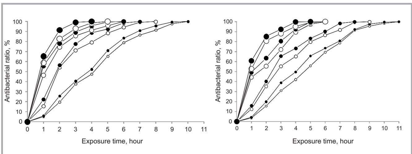
**Figure 11.** Bacteria ratio for (○) 2%, (◐) 4%, (◑) 6%, and (○) 8% of resin concentration for the pad-dry-cure process and (●) 2%, (●) 4%, (●) 6%, (●) 8% of resin concentration for the pad-dry-plasma-cure process for (a) *S. aureus* and (b) *E. coli*.
