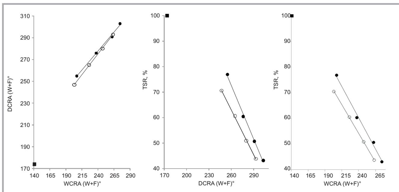
**Figure 5.** Relationships among the: a) DCRA & WCRA, b) TSR & DCRA, and c) TSR & WCRA of the finished fabrics after using (■) the control (○), the pad-dry-cure process, and (●) pad-dry-plasma-cure process, respectively.
