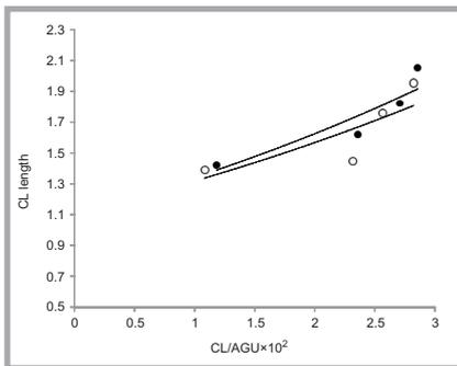
**Figure 7.** Plots of CL length versus CL/AGU of the finished fabrics after using (○) the pad-dry-cure process and (●) pad-dry-plasma-cure process, respectively.
