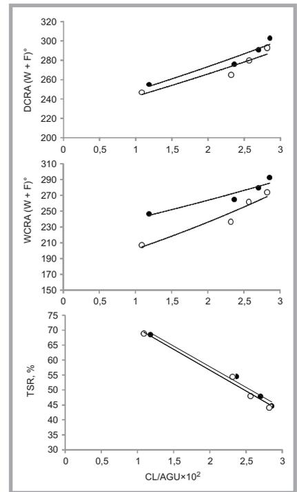
**Figure 8.** Plots of: a) DCRA versus CL/AGU, b) WCRA versus CL/AGU and c) TSR versus CL/AGU of the finished fabrics after using pad-dry-cure process (○) and pad-dry-plasma-cure process (●), respectively.
