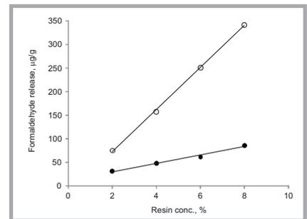
**Figure 9.** Formaldehyde release for DMDHEU-MA crosslinked cotton fabrics versus resin concentration in the pad bath after using (○) the pad-dry-cure process and (●) ad-dry-plasma-cure process, respectively.
