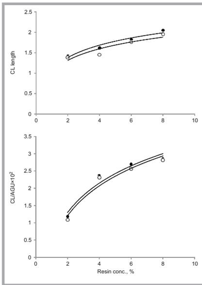
**Figure 6.** Plots of (a) CL length and (b) CL/AGU of the finished fabrics versus resin concentration in the pad bath after using (○) the pad-dry-cure process and (●) pad-dry-plasma-cure process, respectively.
