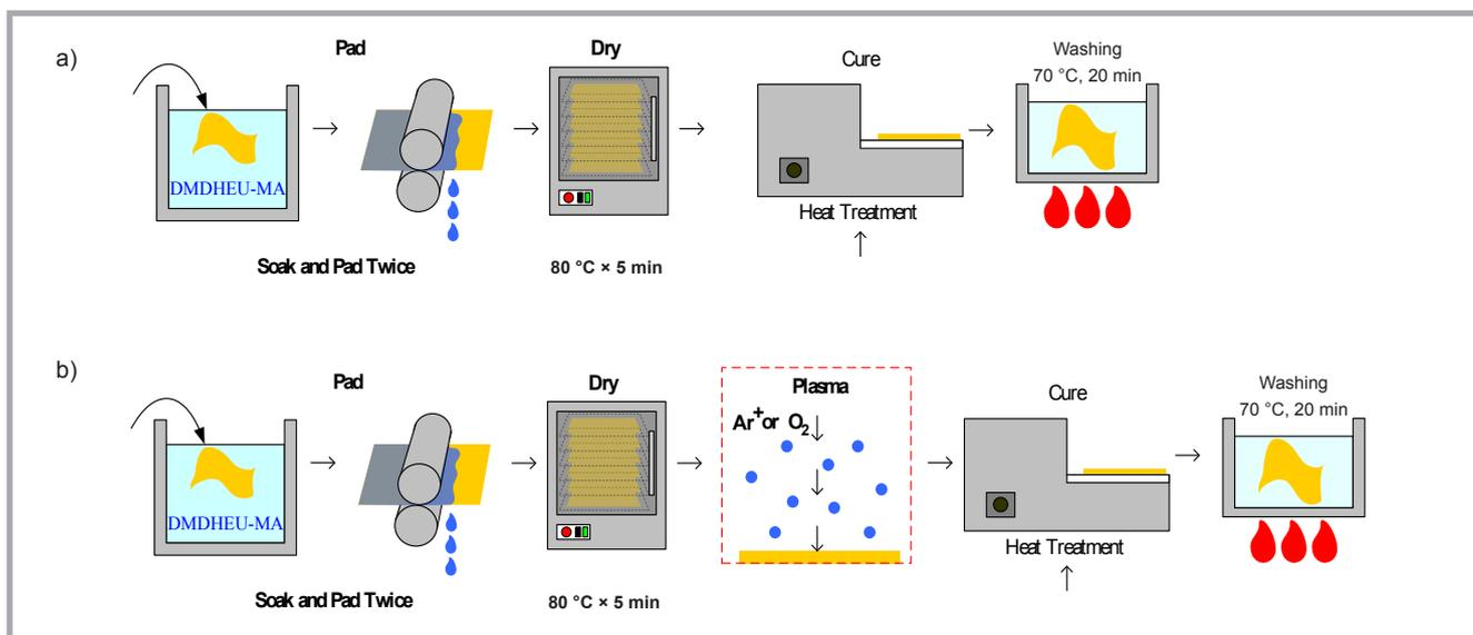
**Figure 1.** a) traditional process, and b) the new process (Plasma treatment is added between the dry and cure of the traditional process).
