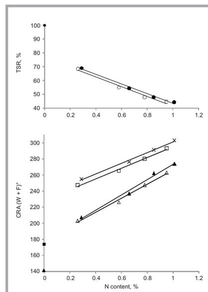
**Figure 4.** Values of TSR, DCRA, and WCRA versus the nitrogen contents of the finished fabrics after using (●, ■, ▲) control, (○, □, △) the pad-dry-cure process, and the (●, ■, ▲) pad-dry-plasma-cure process, respectively.
