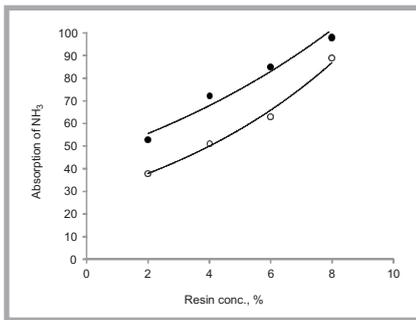
**Figure 10.** Odour absorption for DM-DHEU-MA crosslinked cotton fabrics versus resin concentration in the pad bath after using (○) the pad-dry-cure process and (●) pad-dry-plasma-cure process, respectively.
