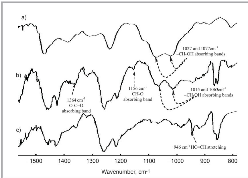
**Figure 3.** FT-IR spectra of (a) DMDHEU, (b) DMDHEU-MA, and (c) MA.
