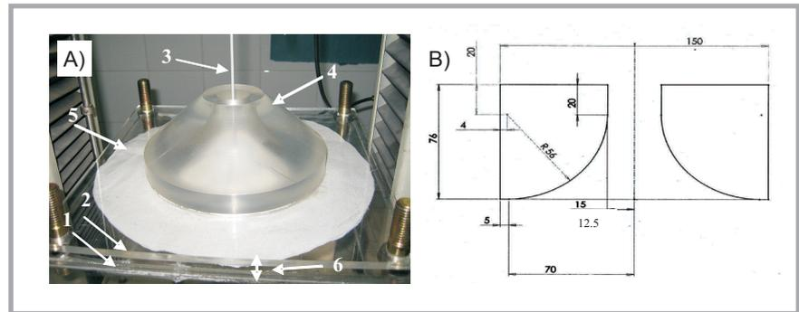
**Figure 2.** A) Pulling through newly designed funnel; 1) base plate, 2) distance plate, 3) pulling axle, 4) funnel, 5) fabric sample, 6) adjustable space. B) Funnel dimensions.
