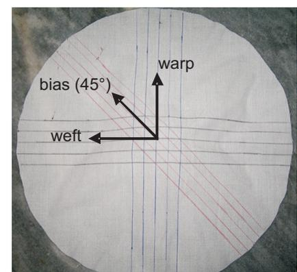
**Figure 3.** Markings on fabric sample in warp, weft and bias directions.
