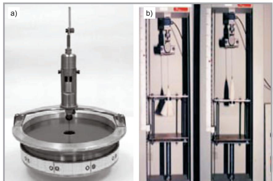
Figure 1. a) pushing through and b) pulling through a ring [11 - 14].
