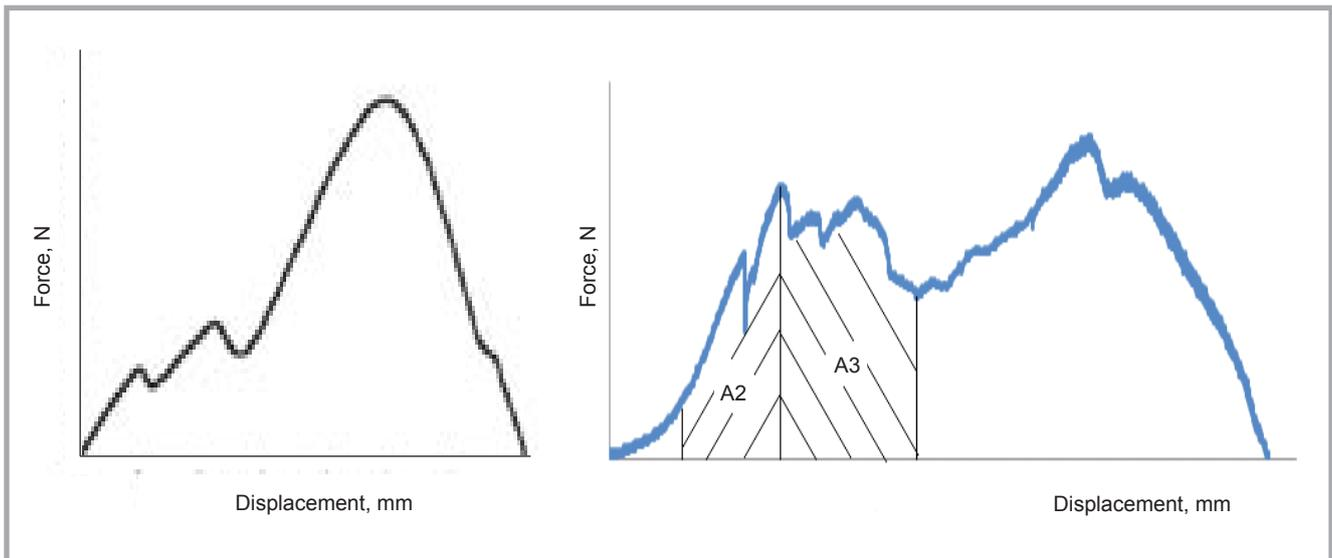
**Figure 5.** Comparison between a known force-displacement curve (A) and that obtained from the new apparatus (B).
