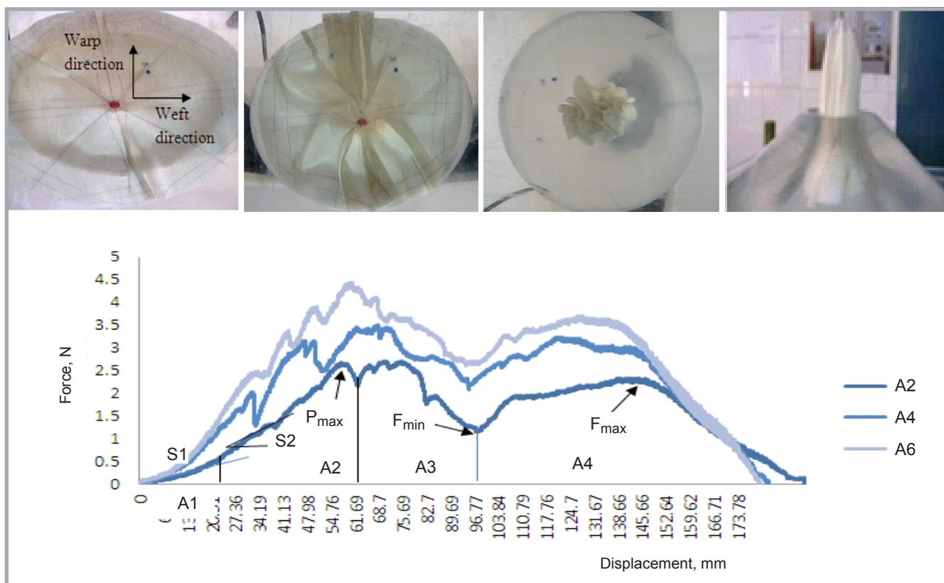
**Figure 4.** Fabric behavior corresponding to different parts of force-displacement curves. A2, A4 and A6: three fabric samples with different weft densities.
