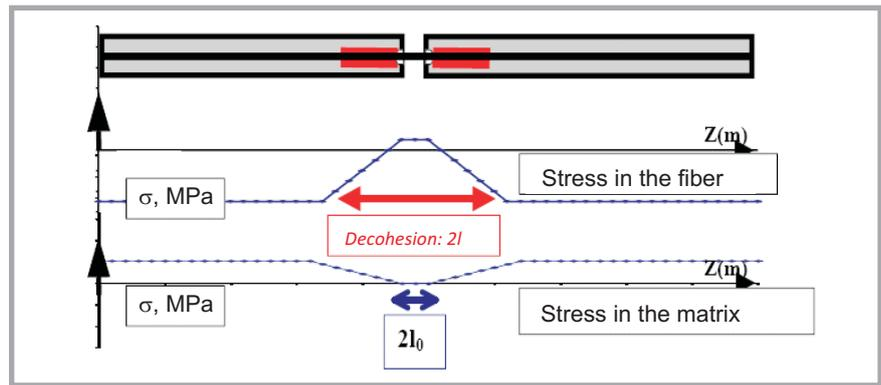
Figure 1. Profile of a constraint in the vicinity of a fibre.
