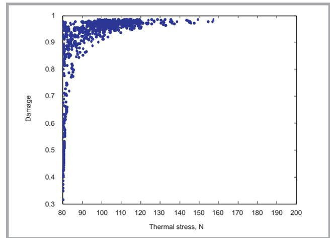
Figure 4. Influence of heat stress on the damage of the matrix.
