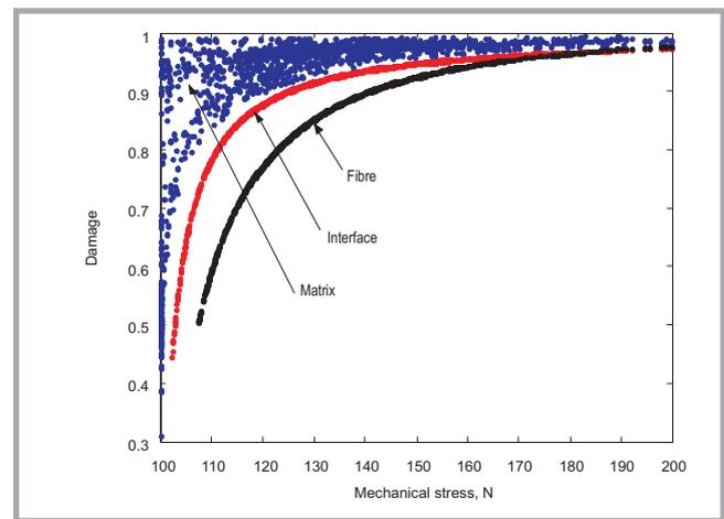
Figure 6. Influence of thermal stress on the damage of the fibre-matrix interface.
