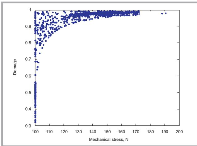
Figure 3. Influence of mechanical stress on the damage of the matrix.
