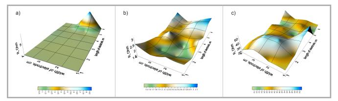
*Figure 6.* Example of the surface resistance distribution on a textile electrode: 1 - electro-conductive silicone foil with silver particles, 2 - woven fabric made of Nitril Static yarn, <math>3 - graphite nonwoven.
