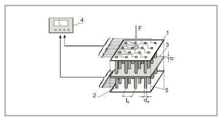
**Figure 5.** Simplified scheme of the volume resistance measurement stand, 1 - upper multipoint measurement probe, <math>2 - lower multipoint measurement probe, <math>3 - textile electrode, 4 - Agillent 6.5 Digits Mullimeter, 5 - crossrails, F - preasure force
