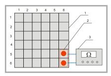
**Figure 4.** Simplified scheme of a stand for measuring surface resistance; 1 – textile electrode, 2 – dual point probes, 3 – Agillent 6.5 Digits Mullimeter.
