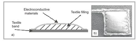
*Figure 1.* Scheme of a textile composite electrode for electrostimulation (a), real photo of the structure (b).
