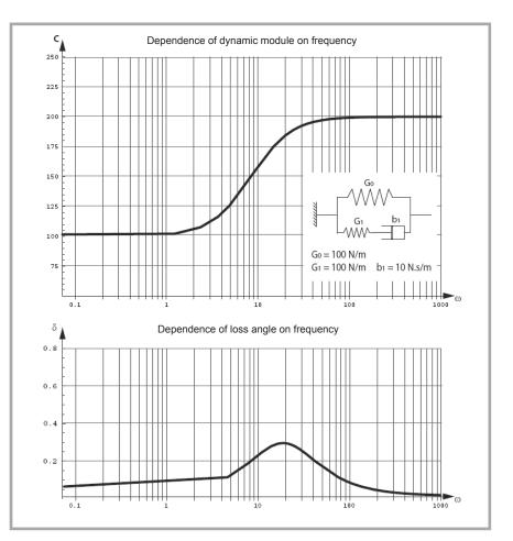
Figure 3. Dynamic characteristics of the three-membered rheological model.
