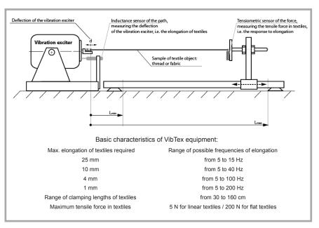
Figure 4. Principle of VibTex equipment.
