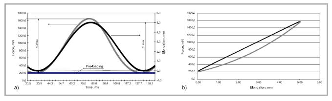
*Figure 5. Example of the result of a test with harmonic elongation: frequency 10 Hz, maximum elongation - 5 mm; a) time dependence of the force and the elongation, b) dependence of the force on the elongation.*
