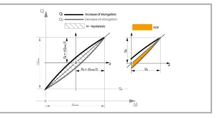
Figure 7. Dependence of the tensile force on elongation.
