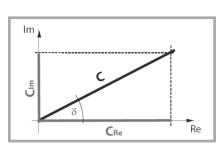
**Figure 1.** Dynamic module of rigidity, its real and imaginary components;  $C = T(i\cdotw) - dynamic module of rigidity,$  $C_{Re} = Re[T(i\cdotw)] - real component (elastic$  $module of rigidity), <math>C_{Im} = Im[T(i\cdotw)]$ imaginary component (elastic module of rigidity)
