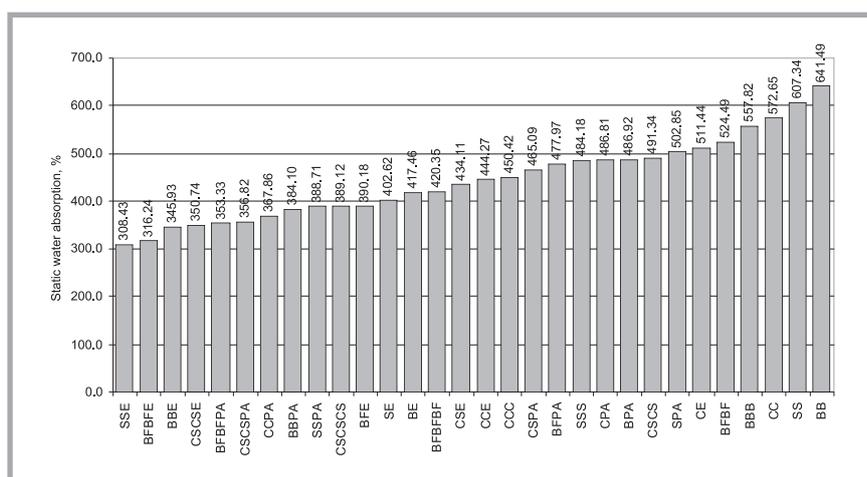
**Figure 1.** Static water absorption of knitted socks samples.
