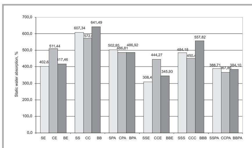
**Figure 2.** Static water absorption of pure knits manufactured from soy, cotton, bamboo (linear density XX-28 tex, XXX-42 tex) and its combination with elastane (XE-24 tex, XXE-38 tex) and textured polyamide (XPA-34tex, XXPA-48 tex) threads.
