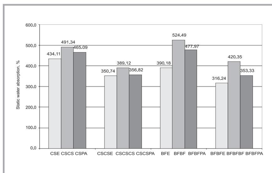
**Figure 3.** Static water absorption of knits manufactured from Cotton – seacell (CSCS-38 tex, CSCSCS-57 tex), combination with elastane (CSE-29 tex, CSCSE-48 tex) and textured polyamide (CSPA-39 tex, CSCSPA-58tex); Bamboo – flax (BFBF-48 tex, BFBFBF-72 tex), combination with elastane (BFE-34 tex, BFBFE-58 tex) and textured polyamide (BFA-44 tex, BFBFA-68 tex) threads.
