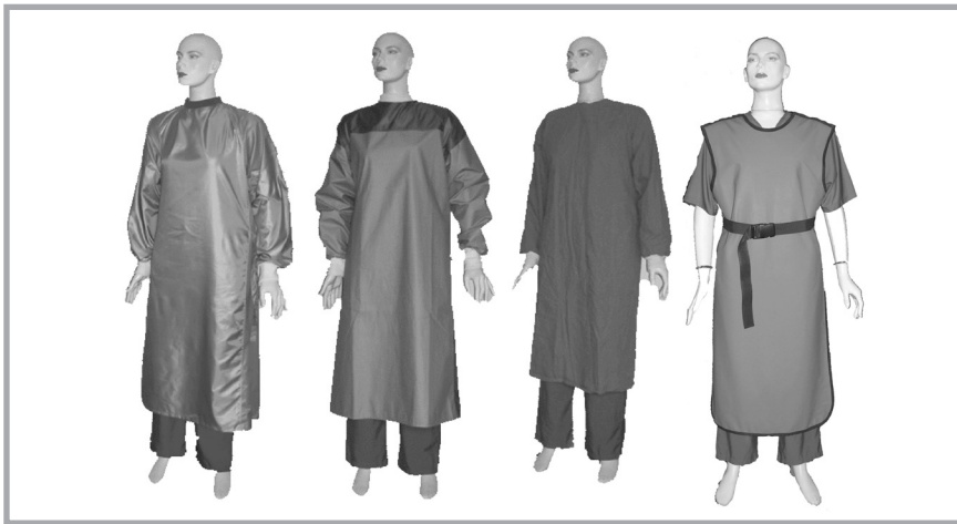
Figure 1. Thermal manikin wearing ensembles of surgical gowns (A – surgical underwear and ensemble A, B – surgical underwear and ensemble B; C - surgical underwear and ensemble C; D - surgical underwear and ensemble D).
