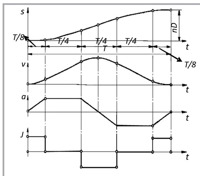
**Figure 2.** The motion rule of trapezoidal acceleration curve.
