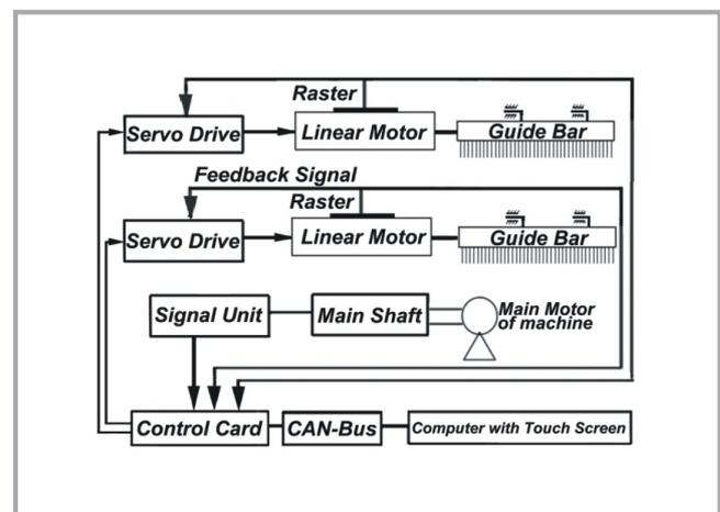
is transmitted to the servo drive and control card by a raster installed in the output axle of the liner motor. The difference between the actual position and enactment will be compensated by the control procedure so that the system can achieve high precision.
