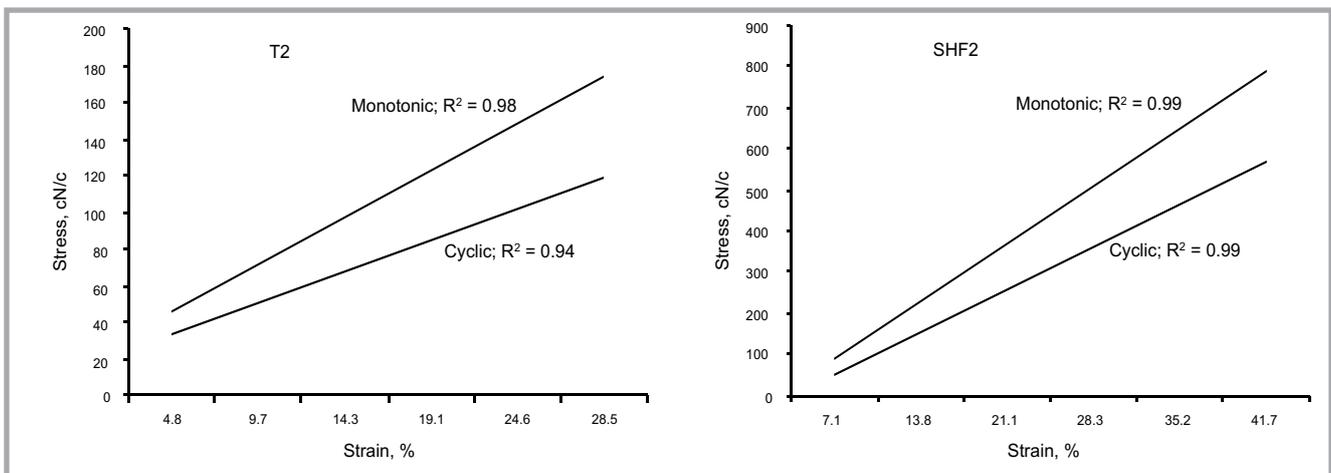
**Figure 6.** Monotonic and cyclically stabilised stress-strain curves for fabric samples  $T_2$  and  $SHF_2$ .
