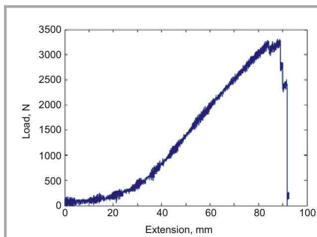
**Figure 2.** Typical load-extension diagram of fabric T2.
