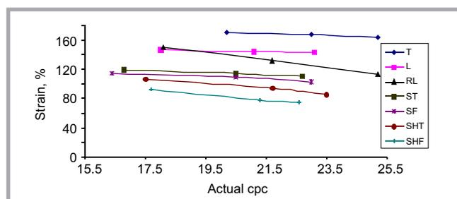
**Figure 3.** Breaking strain of fabrics of different actual  $cpc$ .
