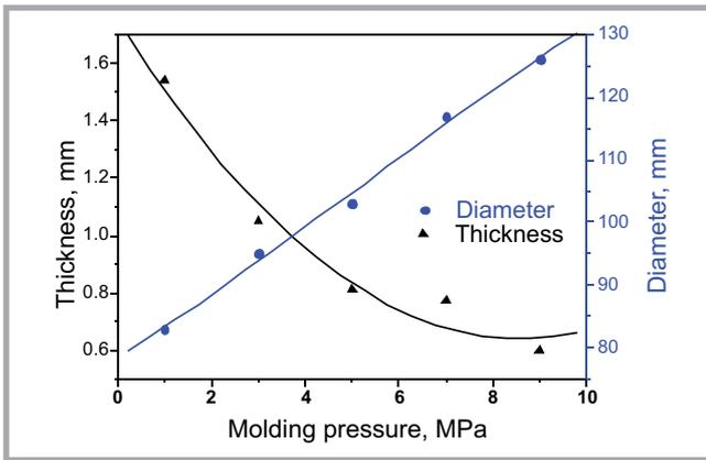
**Figure 7.** Effect of moulding pressure on the plasticity of super-fine wool powder film.
