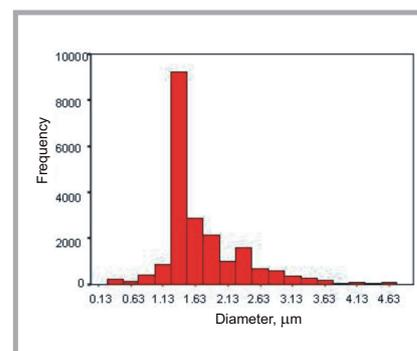
Figure 1. Particle size distribution of superfine wool powder.
