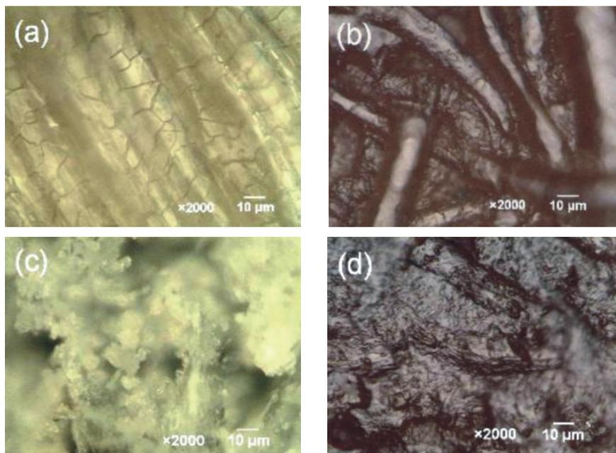
**Figure 2.** Micrographs of hot-pressed films from (a) wool fabric, (b) wool fibres and (d) superfine wool powder, (c) Micrograph of superfine wool powder without hot-pressing.
