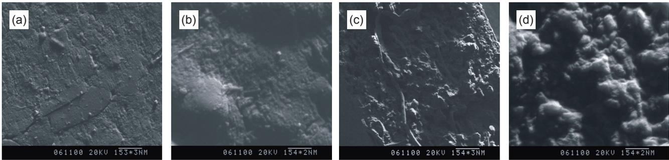
**Figure 4.** SEM photos of thermoplastic films of superfine wool powder: (a), (b): surface morphology; (c), (d): cross-section.
