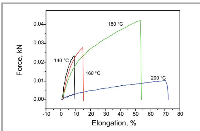
**Figure 9.** Force-elongation curves of thermoplastic films at different moulding temperatures.
