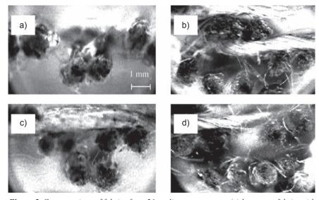
**Figure 5.** Cross-sections of fabrics from 56 tex linen spun yarns: (a) loomstate fabric, with  $S_2 = 210 \text{ dm}^{-l}$ , (b) fabric after laundering, with  $S_2 = 210 \text{ dm}^{-l}$ , (c) loomstate fabric, with  $S_2 = 270 \text{ dm}^{-l}$ , (d) fabric after laundering, with  $S_2 = 270 \text{ dm}^{-l}$ .
