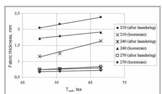
*Figure 7.* Thickness variation of fabric and increasing linear density of wefts, when density of wefts is constant.
