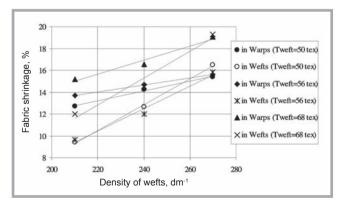
*Figure 3. The dependence of fabric shrinkage after five laundering cycles on weft yarns density.*
