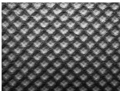
**Figure 2.** PP fabrics with deposited Zn-Bi layer.
