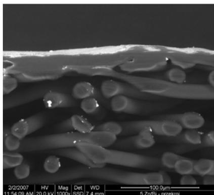
**Figure 3.** SEM image (SEM 1000x) of cross-sections of polypropylene fabric deposited by the DC-M method (a) for  $P = 180$  W, (b) for  $P = 400$  W.
