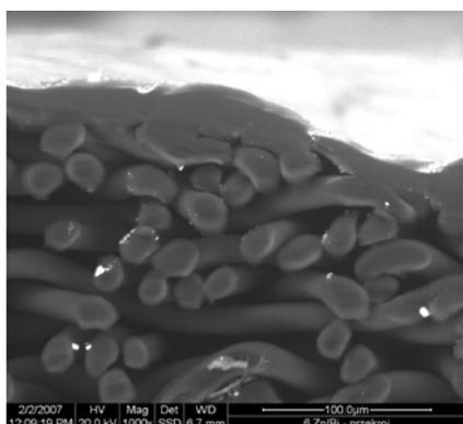
**Figure 4.** SEM image (SEM 5000x) of PP fiber surface obtained by the AC-M method at a low power level,  $P = 180$  W, of the target supply.
