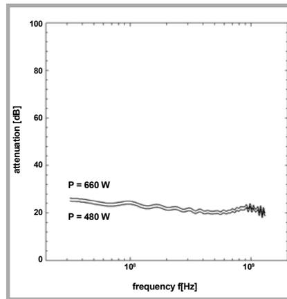
**Figure 8.** Effect of power dissipated in the target on the value of the EM field attenuation of PP fabric coated with a 0.96Zn-0.04Bi metallic layer. Sputtering in the AC-M mode at the group frequency  $f = 5$  kHz.
