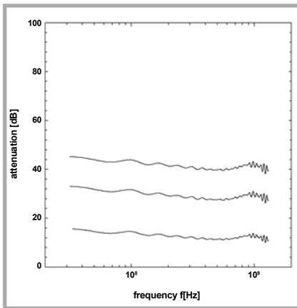
**Figure 7.** Effect of power dissipated in the target on the value of the EM field attenuation of PP fabric coated with a 0.9Zn-0.1Bi metallic layer. Sputtering in the DC-M mode at the group frequency  $f = 5$  kHz.
