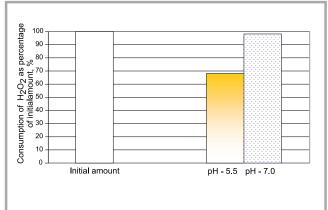
**Figure 4.** Exhaustion of hydrogen peroxide after the bleaching of waste paper with peracetic acid with dependence on the reaction medium; (1% Pa as  $H_2O_2$ , 0.5% MgSO<sub>4</sub>, time 60 min, pulp conc. 20%).
