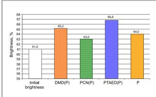
**Figure 9.** Comparison of the two step bleaching effectiveness of dimethylooxsirane (DMD), hydroxy peroxide activated by ammonium molybdate ( $P_{akt}$ ), cyanamide ( $P_{CN}$ ) and TAED ( $P_{TAED}$ ) in the bleaching of waste paper pulp.
