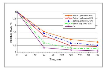
*Figure 1.* Residual  $H_2O_2$  after bleaching at a pulp concentration of 12 and 20% for two waste paper pulp batches with dependence on time; 3%  $H_2O_2$ , 0.2% MgSO<sub>4</sub>, 0.1% EDTA, 0.3% NaOH,  $pH \approx 10.5$ , 90 °C, pulp conc. 12 and 20%.
