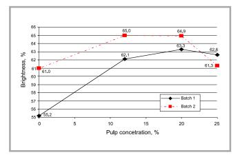
**Figure 3.** Comparison of  $H_2O_2$ , bleaching effectiveness of waste paper pulp with dependence on pulp concentration;  $3\% H_2O_2$ , 0.2% MgSO<sub>4</sub>, 0.1% EDTA, 0.3% NaOH, pH  $\approx$  10.5, 90 °C, 180 min.
