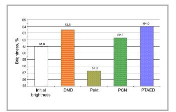
**Figure 8.** Comparison of the bleaching effectiveness of dimethylooxsirane (DMD), hydroxy peroxide activated by ammonium molybdate ( $P_{akt}$ ), cyanamide ( $P_{CN}$ ) and TAED ( $P_{TAED}$ ) in the bleaching of waste paper pulp.
