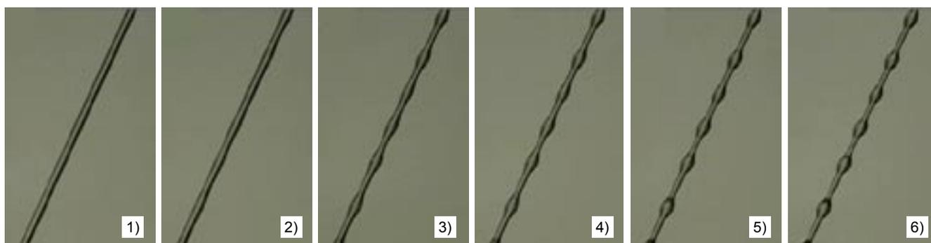
Figure 3. Development of PVA film instability on polyamide fibre inclined at 70°: pictures (1) – (6) were taken every 0.5 sec.
