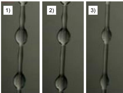
**Figure 6.** Representation of droplet flattening as a function of time on the Polyamide filament inclined by 90°.
