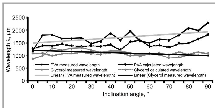
**Figure 4.** Comparison of measured and calculated wavelengths between PVA and glycerol droplets.
