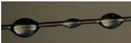
**Figure 5.** Arrangement of mother and daughter droplets at an inclination angle of 5°.
