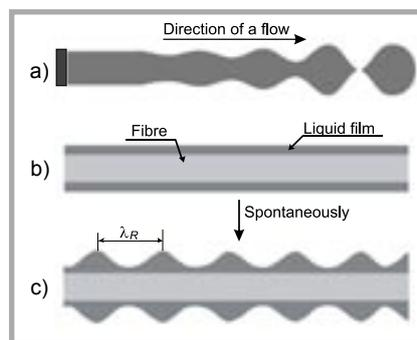
Figure 1. a) The formation of the instability of the jet [2]. b) and c) The formation of liquid film instability [3].
