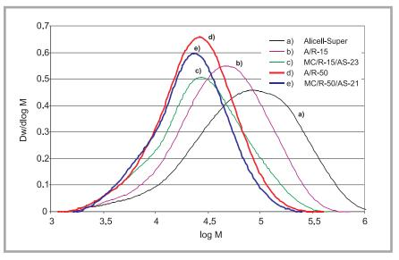
*Figure 3.* Molecular weight distribution curves of cellulose pulp and MCC obtained with two-step radiation/ enzymatic degradation.
