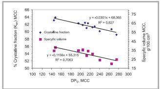
*Figure 2.* Dependence of crystalline phase content and specific volume of MCC on its average polymerisation degree.
