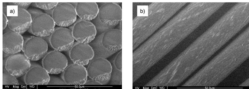
**Figure 2.** SEM photos of DBC fibres solvent - DMSO; a) cross-section, b) surface.
