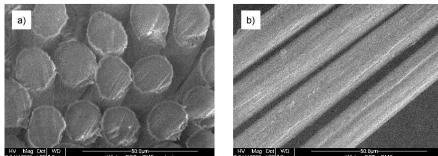
**Figure 1.** SEM photos of DBC fibres solvent - DMF; a) cross-section, b) surface.
