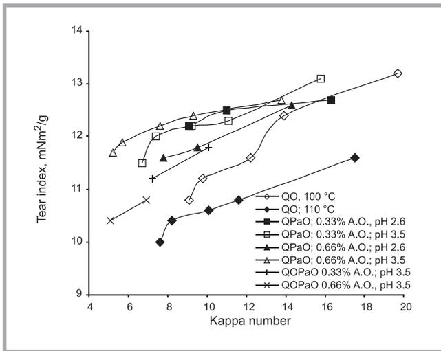
**Figure 3.** Relationship between tear index and kappa number of oxygen-delignified pine kraft kappa number 31.5 pulp in different variants of the process. (Standard deviation of tear index measurements was  $0.2 \text{ mN} \cdot \text{m}^2/\text{g}$ ).
