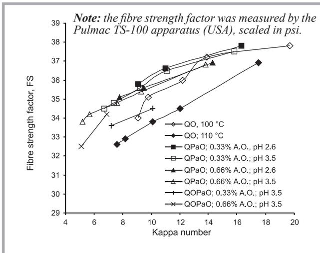
**Figure 5.** Relationship between zero-span fibre strength factor and kappa number of oxygen-delignified pine kraft kappa number 31.5 pulp in different variants of the process (after beating the pulp in a Jokro mill to freeness  $20^\circ\text{SR}$ , beating time 12 min.); (Standard deviation of FS-factor was 1.1).
